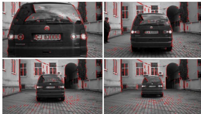
Fig. 3.3. The re-projection result of the 3D points onto the left image of the stereo-pair: top-left – the car is at 2 m; top-right – the car is at 4 m; bottom-left – the car is at 6 m; bottom-right – the car is at 8 m.
