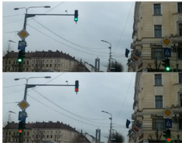
Fig. 3.6. Result of color threshold segmentation for the green traffic lights present on the top image. Detected green pixels are marked with red, on the bottom image
