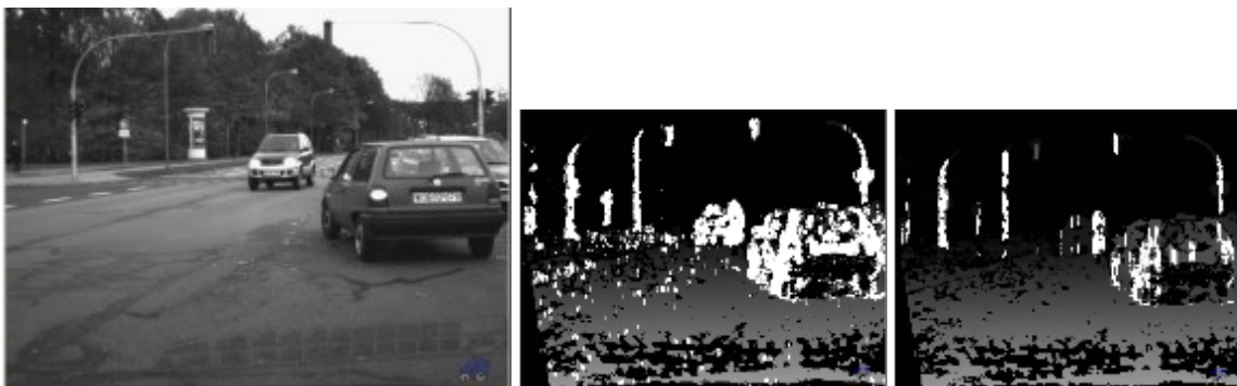
Fig. 4.3. If the threshold applied on the u-disparity map is not adapted with the depth, then noise remains if its value is too low, or most of the obstacle pixels are missed, if too high.
