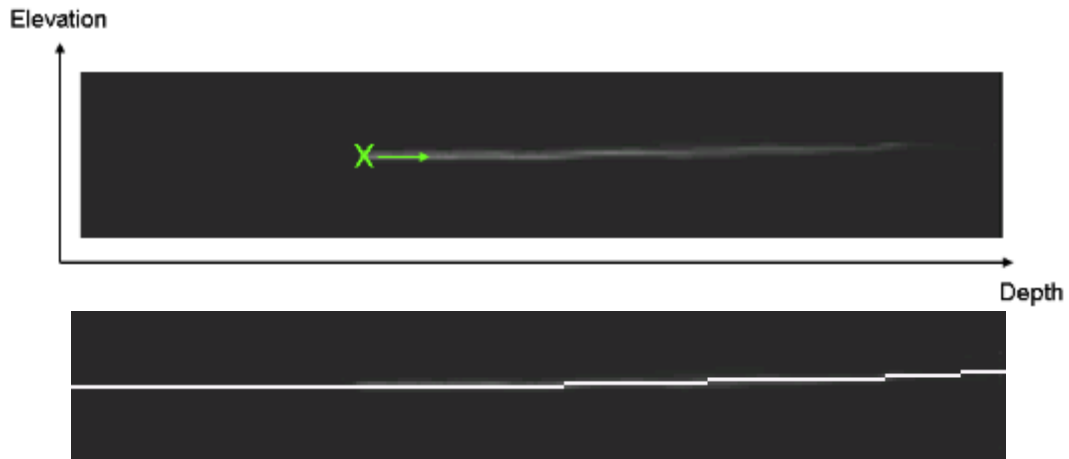
Fig. 5.11. Top: the road profile is searched in the histogram space from the starting point towards larger depths; bottom: the extracted road profile, extended back toward the ego car
