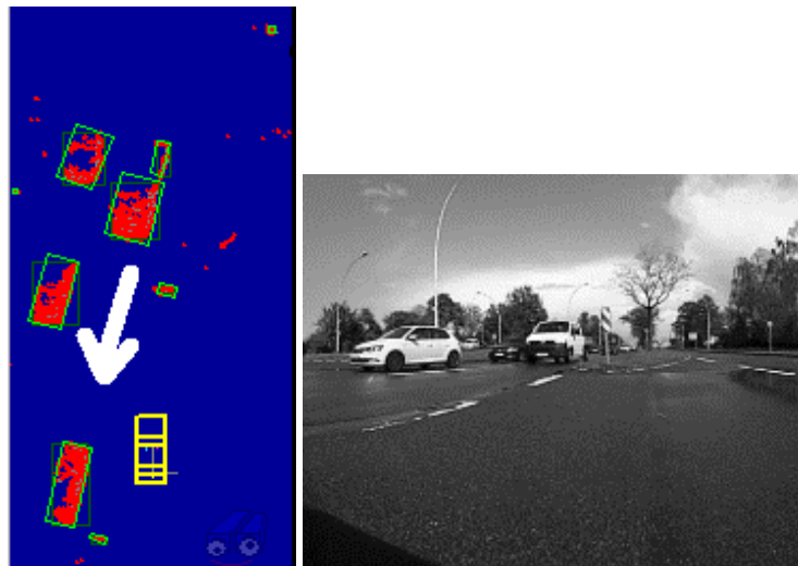
Fig. 6.10. Scenario 1 used for evaluation. Incoming traffic (the direction of motion shown with the white arrow) at an angle of 14.4 degrees
