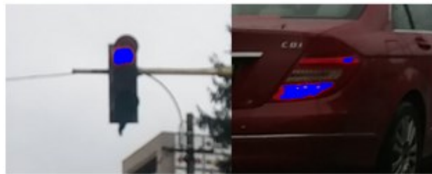
Fig. 3.7. Red traffic light and false detection on car tail lights (detected red pixels marked blue)
