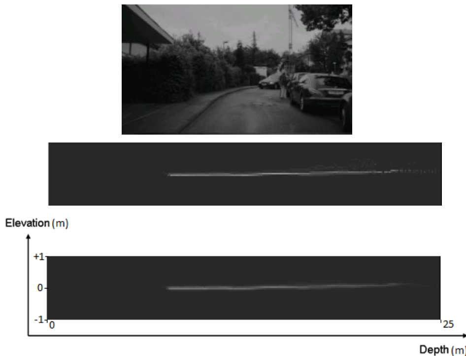
Fig. 5.10. Top: left image; middle: the search space used for road profile estimation, on each column the intensity encoding of the histogram of elevations is shown; bottom: the search space after Gaussian smoothing
