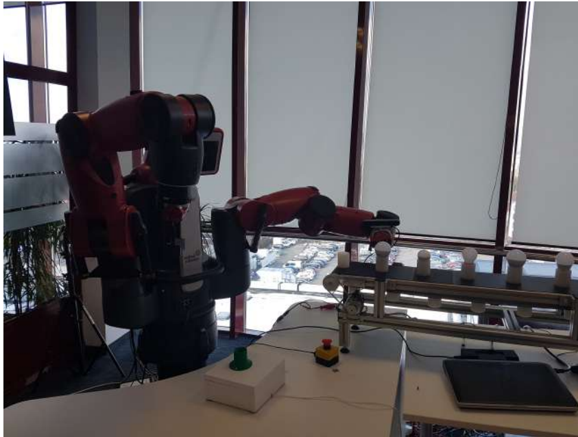
Figure 5.14: A real robot performing the sorting of light bulbs
