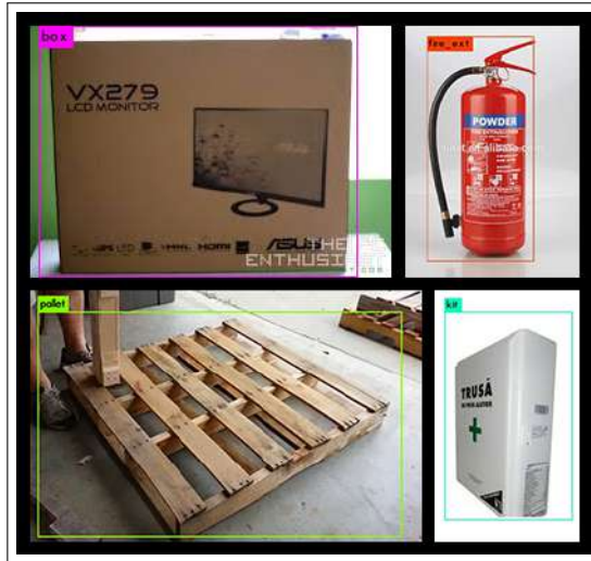
Figure 3.5: Examples of detection of the objects of interest, after applying the trained model, using Darknet Redmon (2013–2016) and the modified YOLOv2 Redmon & Farhadi (2016) network.
