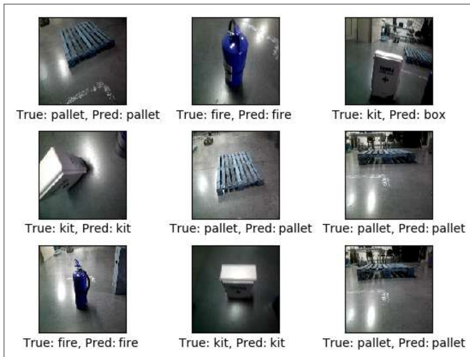
Figure 3.7: The correct and predicted labels of nine, randomly chosen objects from the list. True - real label, Pred - predicted label.
