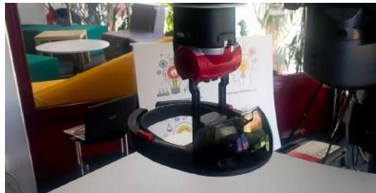
Figure 5.24: Calibration procedure with Baxter and HoloLens
