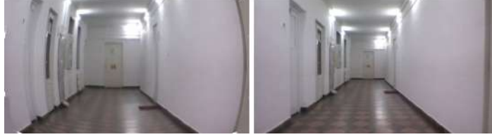
Figure 5.4: Camera calibration, on the left the barrel distorted image, on the right the calibrated image.
