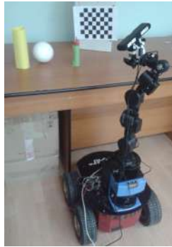
Figure 5.9: The 7DoF robot arm model with the 3D depth sensor mounted on the top of it
