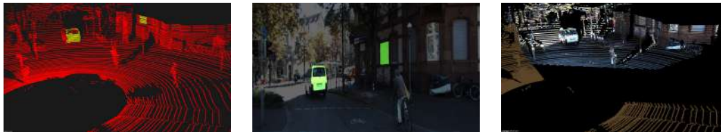
Figure 4.5: Calibration example with real data of an outdoor environment (left-right): 3D data with the selected region (yellow); color 2D data with the corresponding region (green); color information overlaid on 3D data using the extrinsic parameter estimates
