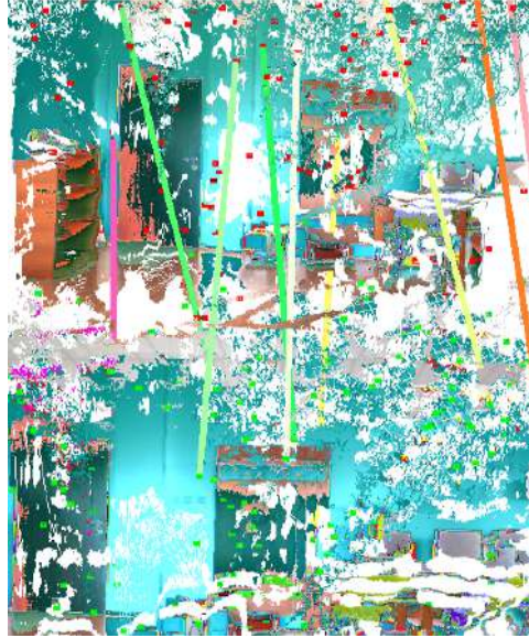
Figure 2.3: Feature matching for coloured point cloud from stereo camera with Daisy algorithm
