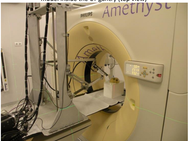
f) Needle insertion inside the tumour under CT real-time control
