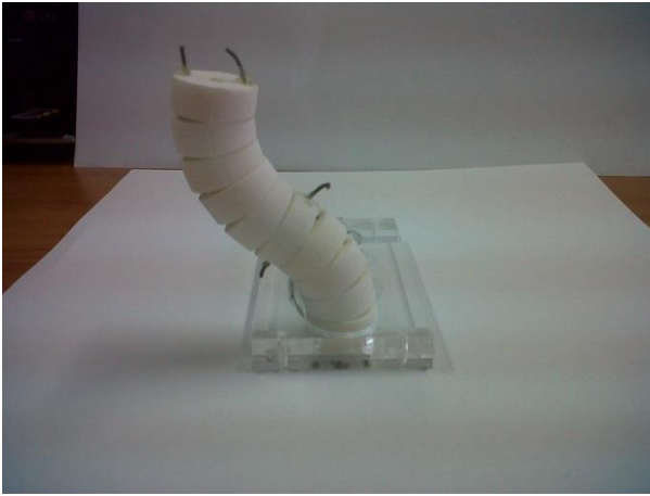
Figure 2.28. Module with both bends actuated
