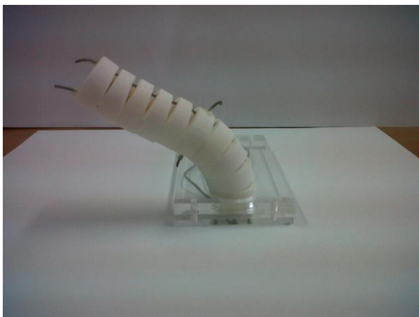
Figure 2.26. Module with first bend actuated and second one straight
