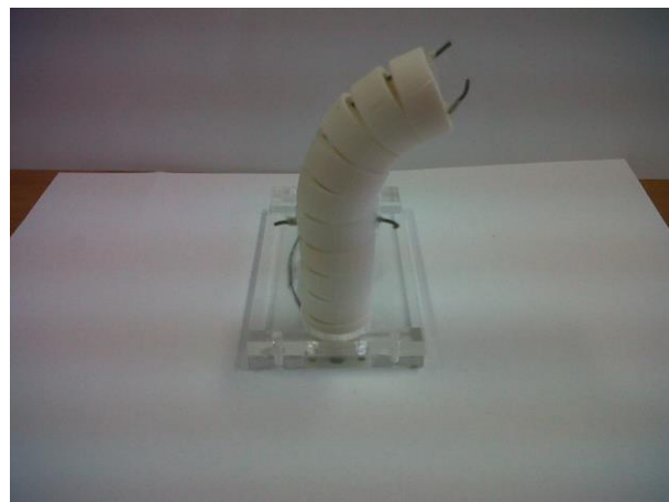
Figure 2.27. Module with first bend non-actuated and second one actuated
